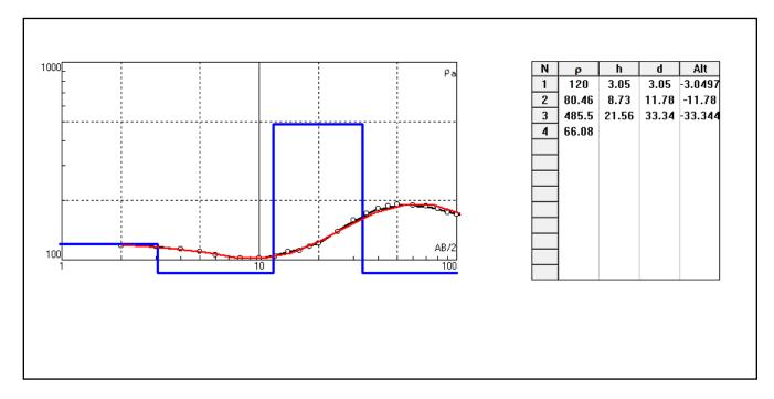
Fig-6.3: VES Curve and interpreted results at Badadhara (Near Urja Road, Inside plant area) (VES 1)
