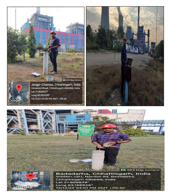
Fig 7.2: Piezometric Point for Ground water level Monitoring in the plant area
